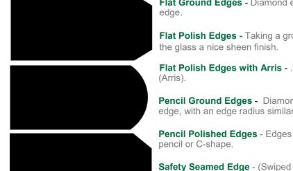
Flat Ground Edges - Diamond embedded grinding wheels put a satin finish on the
